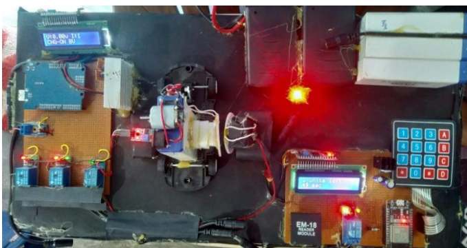
fig. d. Hardware Implementation of RFID based Wireless EV charging system
